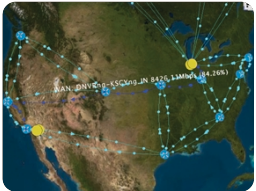
Figure 3: The MonALISA framework provides a distributed monitoring service system. Each MonALISA server acts as a dynamic service system and provides the functionality to be discovered and used by any other services or clients that require such information.
